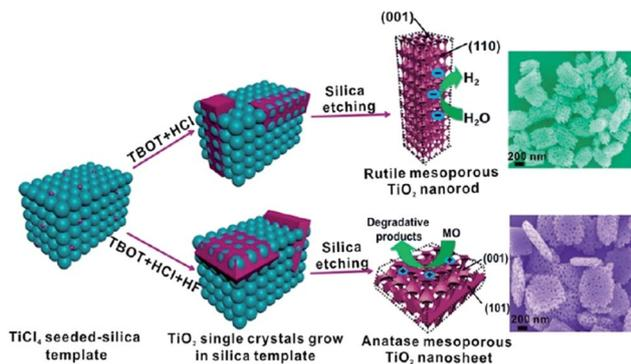
Fig. 5 Schematic illustration of the synthesis pathways of rutile  $\text{TiO}_2$  mesocrystals and anatase  $\text{TiO}_2$  mesocrystals using silica templates by a hydrothermal method. Adapted with permission from ref. 61. Copyright 2013 American Chemical Society.
