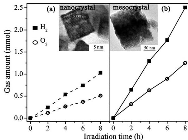
**Fig. 14** Photocatalytic water splitting for hydrogen and oxygen generation. (a) Nanocrystals (dashed line) and (b) NaTaO<sub>3</sub> mesocrystals (solid line). Adapted with permission from ref. 101. Copyright 2013 Elsevier.
