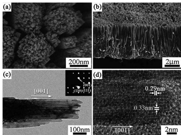
Fig. 6 (a and b) SEM, (c) TEM, and (d) HRTEM images of rutile  $\text{TiO}_2$  nanorod arrays prepared at 150 °C on Ti foil for 20 h. The inset in (c) is the corresponding SAED pattern. Adapted with permission from ref. 64. Copyright 2012 Royal Society of Chemistry.
