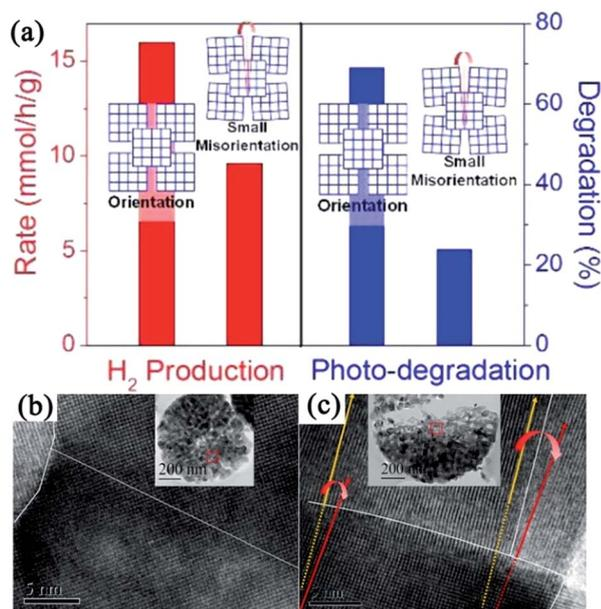
Fig. 4 (a) Schematic illustration of disordered and ordered aggregations of TiO<sub>2</sub> nanoparticles and their corresponding photocatalytic activities. (b) HRTEM image of TiO<sub>2</sub> mesocrystal with oriented orientation. (c) HRTEM image of TiO<sub>2</sub> mesocrystal with misorientation (crystal lattice mismatch). Adapted with permission from ref. 53. Copyright 2015 American Chemical Society.
