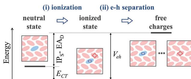
Fig. 5 Illustration of the elementary steps of the p-doping process for a generic molecular semiconductor and of the electronic states involved with their relative energies.  $IP_S$ ,  $EA_D$  and  $E_{CT} = IP_S - EA_D + V_{eh}$  do all refer to the adiabatically relaxed values. The dopant molecule in the host OSC is depicted in light blue.
