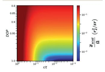
Fig. 4 Average scattering cross section  $\bar{\sigma}_{\text{scat}}$  with respect to the DOP of primary X-rays and the ratio of capillary radius r to collimator plate thickness t. Scattering cross section is in the units of  $r_e^2$ , where  $r_e$ denotes the classical electron radius and equals 2.82  $\times$   $10^{-5}$  Å, and is normalized by the effective solid angle  $\Omega$  of capillaries.
