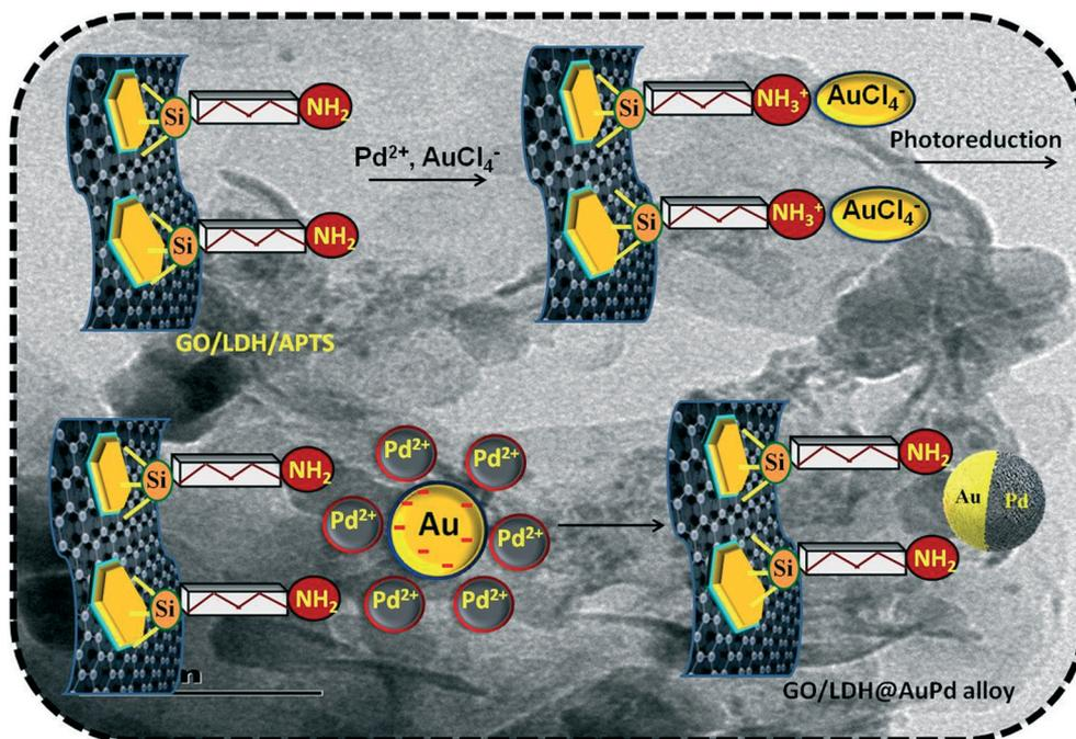
Scheme 1 Mechanism of the formation of the GO/LDH@AuPd photocatalyst.
