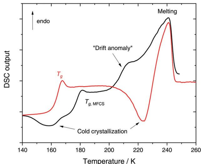
Fig. 8 DSC heating scan at 1 bar ( $30 \text{ K min}^{-1}$ ) of a glassy  $x = 0.20$  glycerol solution vitrified at  $30 \text{ K min}^{-1}$  and ambient pressure (red curve) or produced by pressure-induced amorphization at 77 K (black curve).
