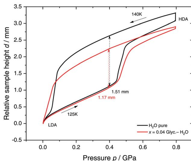
**Fig. 11** Sample height changes upon decompression of HDA (140 K) and compression of LDA (125 K) for 300  $\mu$ L  $x = 0.04$  glycerol-water solution (red curve) and 300  $\mu$ L pure water (black curve). The step height in glycerol-H<sub>2</sub>O is reduced by  $\approx 23\%$  compared to pure water as indicated by the double-headed arrows. Cylindrical samples of 8 mm in diameter were prepared by PIA at 77 K followed by annealing at high pressures.
