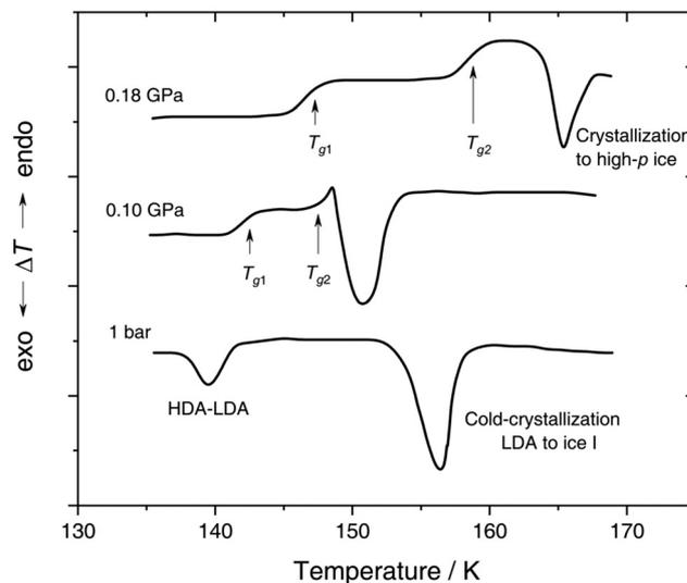
Fig. 4 *In situ* DTA scans of  $x \approx 0.05$  ( $R = 20$ ) LiCl–H<sub>2</sub>O solution vitrified at 0.25 GPa with  $q_c \approx 180$  K min<sup>-1</sup>, then reheated at various pressures with a scanning rate of 8 K min<sup>-1</sup>. The figure is adapted from ref. 132.
