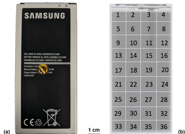
Fig. 1 (a) Photograph of the Samsung J5 cell used throughout the experiments and (b) identification matrix used to identify the locations described in this work overlaid on a radiograph of the J5 cell.
