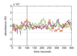
Fig. 4 Mechanical stability of the device is tested by repeated 1 m drop tests. Traces (n=3) show the baseline absorbance before and after impact. The grey vertical bar indicates the approximate time at which the device is released and impacts the floor. No change in baseline absorbance mean or variance is observed as a result of the drop tests.
