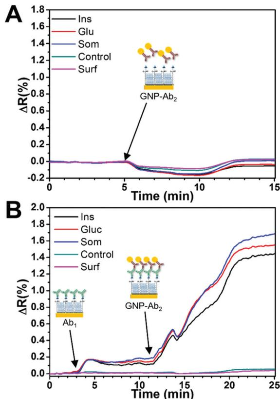
Fig. 5 Real-time SPR angle shift sensorgrams of (A) the nonspecific binding effect of GNP-Ab<sub>2</sub> conjugates and (B) the specific binding effect of GNP-Ab<sub>2</sub> conjugates after primary antibody injection (blank injection  $C_0$ ). Immobilized BSA and the bare SAM surface identified as "Control" and "Surf" were used as negative controls.
