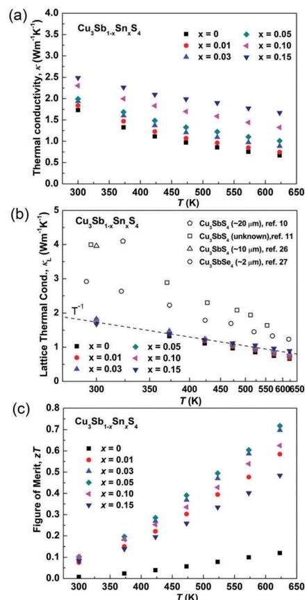
Fig. 8 (a) Thermal conductivity, (b) lattice thermal conductivity and (c)  $zT$  values of as functions of temperature in  $\text{Cu}_3\text{Sb}_{1-x}\text{Sn}_x\text{S}_4$  system.
