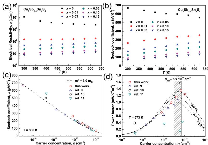
Fig. 5 (a) Electrical resistivity and (b) Seebeck coefficient as functions of temperature; (c) Seebeck coefficient and (d) power factor as functions of carrier concentration in  $\text{Cu}_3\text{Sb}_{1-x}\text{Sn}_x\text{S}_4$  system.
