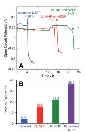
Fig. 7 (A) Open circuit potential as a function of time for uncoated and NHP-coated NZSP pellets with a silver back electrode immersed in 10 M KOH at 80  $^{\circ}$ C. (B) Comparison of lifetimes of NZSP pellets with various NHP coatings subjected to 10 M KOH at 80  $^{\circ}$ C.
