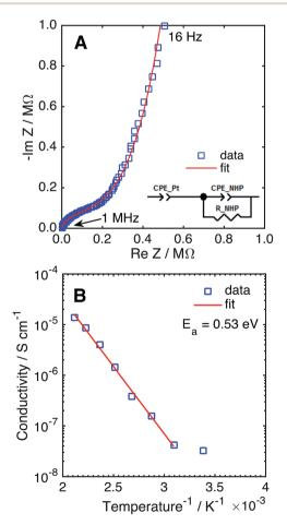
Fig. 6 (A) Nyquist plot of NHP thin film in a Pt-NHP-Pt structure at  $25~^{\circ}$ C. (B) Na $^{+}$  conductivity of a NHP thin film as a function of temperature.
