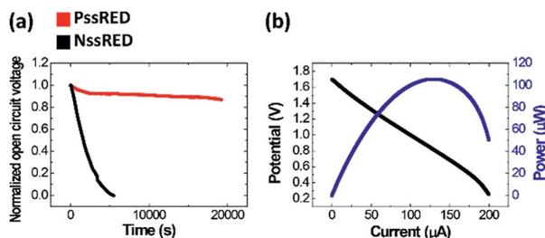
Fig. 2 (a) Normalized open circuit potential (OCP)–time curve of a 4-stack PssRED (red) and normalized OCP–time curve of the NssRED (black). (b) Power (blue) and potential (black) curve of a 20-stack PssRED versus operating current.
