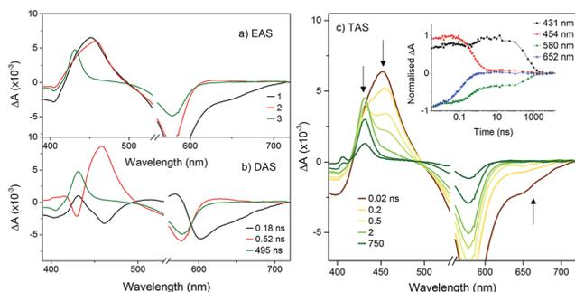
Fig. 4 Transient absorption spectra of  $K_{Sn}^{Mo}[BOD_2]$  in DCM following excitation at 540 nm: (a) evolution associated difference spectra and; (b) decay associated difference spectra derived from global analysis; (c) transient absorption difference spectra at selected time delays after excitation, with single-point decays at 431 nm, 454 nm, 580 nm and 652 nm (inset).
