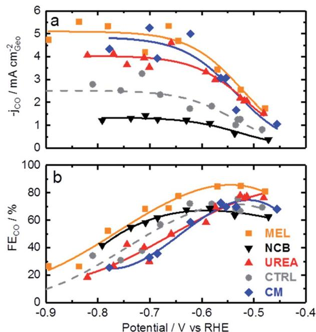
Fig. 4  $\text{CO}_2$  reduction data for various Fe–N–C catalysts based on different secondary nitrogen precursors: (a) CO generation rate, (b) faradaic efficiency towards CO production. Experimental conditions:  $\text{CO}_2$  saturated 0.1 M  $\text{KHCO}_3$ , catalyst loading:  $0.75 \text{ mg cm}^{-2}$  on glassy carbon.
