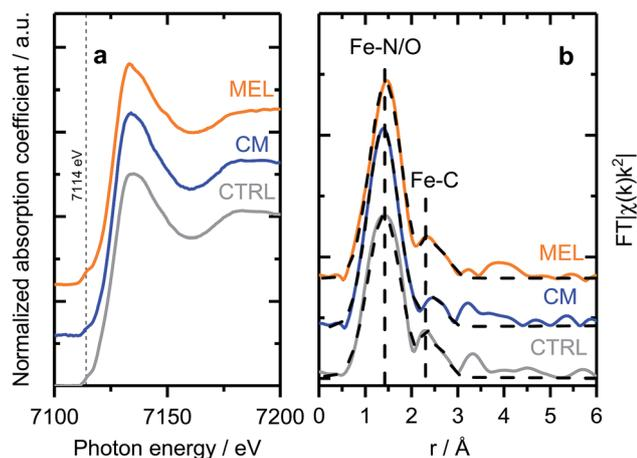
Fig. 3 (a) Fe K-edge XANES and (b) EXAFS spectra of selected Fe–PANI samples, dotted lines in (b) show fitted models.
