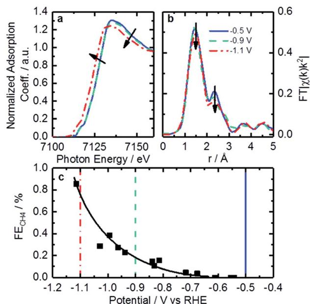
Fig. 7 Fe K-edge XANES (a) and EXAFS (b) spectra taken under *operando* conditions in  $\text{CO}_2$ -saturated  $0.1 \text{ M KHCO}_3$  at  $-0.5$  V (solid blue curves),  $-0.9$  V (dashed green curves) and  $-1.1$  V (red dot-dashed curves) vs. RHE. (c) Faradaic efficiency to  $\text{CH}_4$  varying with potential. Lines are added to indicate points representative of spectra in (a) and (b).
