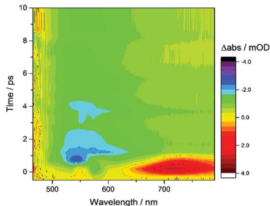
Fig. 6 TA spectroscopy of ZnSe-BF<sub>4</sub>/MEDA (0.5 μM ZnSe-BF<sub>4</sub>, 25 μM MEDA) in aqueous solution in the presence of AA (0.1 M, pH 6.5, Ar, room temperature), showing the first 10 ps following excitation (400 nm).
