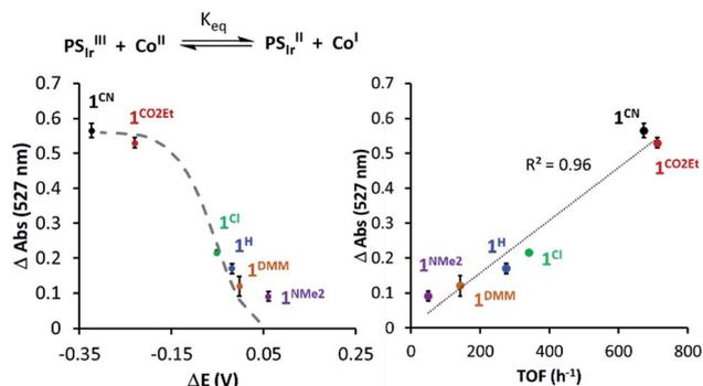
Fig. 7 (Left) The 527 nm absorbance decay upon addition of  $1^{\text{R}}$  vs.  $\Delta(E_{1/2}(\text{PSIr}^+/\text{PSIr}) - E_{1/2}(\text{Co}^{\text{II/I}}))$ . (Right) 527 nm absorbance of  $\text{PSIr}$  decay upon addition of  $1^{\text{R}}$  vs.  $\text{TOF}$  ( $\text{h}^{-1}$ ) (initial rate at 10% conversion of  $\text{H}_2$  evolution). The dashed grey line refers to the theoretical values predicted from Nernst equation (see Section ESI 6.1†).
