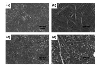
Fig. 3 SEM images of the BC and BCC<sub>60</sub> composites (a) BC, X 30k; (b) BC, X 100k; (c) BCC<sub>60</sub>, X 30k; (d) BCC<sub>60</sub>, X 100k.
