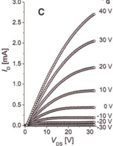
Fig. 4 The plot of drain current  $I_{\rm D}$  versus drain-source voltage  $V_{\rm DS}$  as a function of the gate voltage  $V_{\rm G}$  for an FET nanocrystal with a channel composed of 8 nm PbSe nanocrystals treated with hydrazine solution for 12 hours. Adapted with permission from ref. 47.
