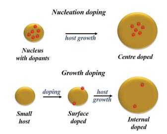
Fig. 5 Schematic of the proposed radial positions of the dopant in nucleation- and growth-doping.
