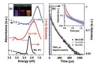
Fig. 13 (a) Steady-state PL (solid line) and absorption (dashed line) of  $\mathrm{Ni}^{2+}$  (blue),  $\mathrm{Co}^{2+}$  (red) and  $\mathrm{Mn}^{2+}$  (black)-doped QDs. (b) Lifetime decay plots for  $\mathrm{Ni}^{2+}$ ,  $\mathrm{Co}^{2+}$  and  $\mathrm{Mn}^{2+}$ -doped CdS collected at the maxima of the broad dopant peaks. The inset of (b) shows the enlarged portion of the lifetime decay of the  $\mathrm{Ni}^{2+}$  and  $\mathrm{Co}^{2+}$ -doped CdS. Adapted from ref. 43.
