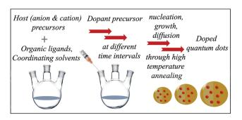
Fig. 1 Schematic of the general colloidal synthesis of organic ligandcapped doped quantum dots.
