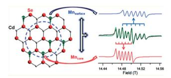
Fig. 14 Theoretical fit and deconvolution of the 406.4 GHz HF-EPR spectra allowing assignment of discrete sites for Mn<sup>2+</sup> occupying a substitutional Cd<sup>2+</sup> site within the core (red) and surface (blue). Adapted with permission from ref. 37.
