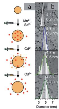
**Fig. 9** TEM images of Mn-doped CdSe. Adapted with permission from ref. 30.
