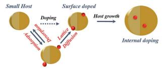
Fig. 2 Schematic of temperature-dependent dopant lattice diffusion.
