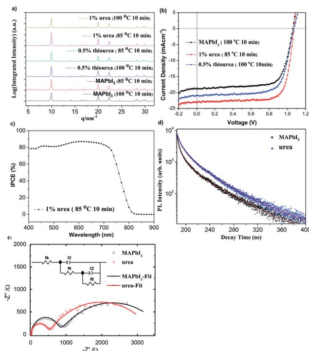
Fig. 3 (a) GIWAXS patterns, (b)  $J$ - $V$  curves, (c) IPCE, (d) TRPL decay curves and (e) electrochemical impedance spectral (EIS) Nyquist plots (the symbols are experimental data, the solid curves are fitting data and the corresponding electronic circuit is shown on top inset) for MAPbI<sub>3</sub> PSCs.
