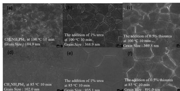
Fig. 2 FE-SEM images of MAPbI<sub>3</sub> perovskite thin films under different conditions (a) MAPbI<sub>3</sub>, (b) 1% urea, (c) 0.5% thiourea at 100 °C for 10 min, respectively; (d) MAPbI<sub>3</sub>, (e) 1% urea, (f) 0.5% thiourea at 85 °C for 10 min, respectively, (scale bar 100 nm).
