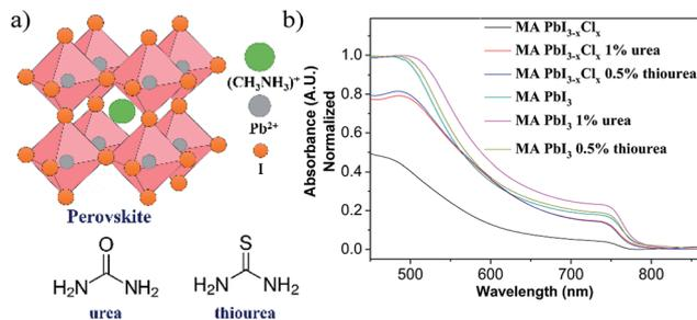
Fig. 1 (a) Chemical structure of perovskite, urea and thiourea (b) UV-vis absorption spectra of perovskites with and without additives.
