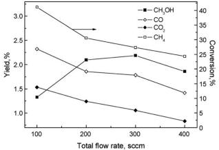
Fig. 2 The effect of flow rate on product distribution (140 W, 7 kHz, 0.5 mm gap distance, ambient temperature, 1 bar, 1:1 CH<sub>4</sub>: O<sub>2</sub>). Reproduced from ref. 107 with permission from Elsevier, copyright 2009.
