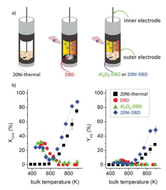
Fig. 6 (a) Reaction environments for the  $CH_4$  reforming and (b) profiles of  $CH_4$  conversions ( $X_{CH_4}$ ) and  $H_2$  yields ( $X_{H_2}$ ) at various reaction environments obtained *via* bulk temperature controls. Reproduced from ref. 200 with permission from American Chemical Society, copyright 2016.
