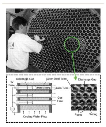
Fig. 9 Assembly of smaller reactor bundles for the industrial scale plasma scale processing (top) and the enlarged view of smaller reactor (bottom). Reproduced from ref. 246 with permission from Springer Nature, copyright 2003.
