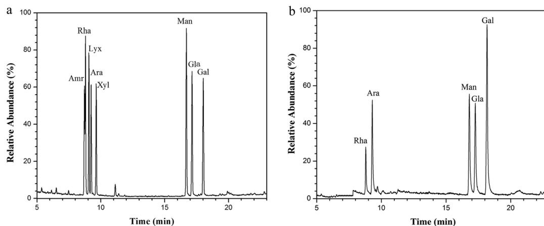
Fig. 4 The GC-MS chromatograms of derivatives of 8 standard monosaccharides (a) and component monosaccharides released from NTWP-II (b). Peaks: (1) D-Amr, (2) L-Rha, (3) D-Lyx, (4) D-Ara, (5) D-Xyl, (6) D-Man, (7) D-Gla, (8) D-Gal.
