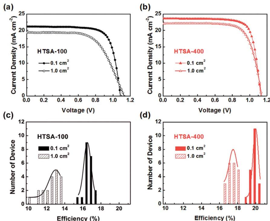
Fig. 19 (a) Current–voltage curves of perovskite solar cells derived from HTSA-100 and (b) HTSA-400 with an active area  $0.1 \text{ cm}^2$  and a  $1 \text{ cm}^2$ . (c) Histogram of PCEs derived from HTSA-100 and (d) HTSA-400 with an active area  $0.1 \text{ cm}^2$  and  $1 \text{ cm}^2$ .<sup>35</sup>
