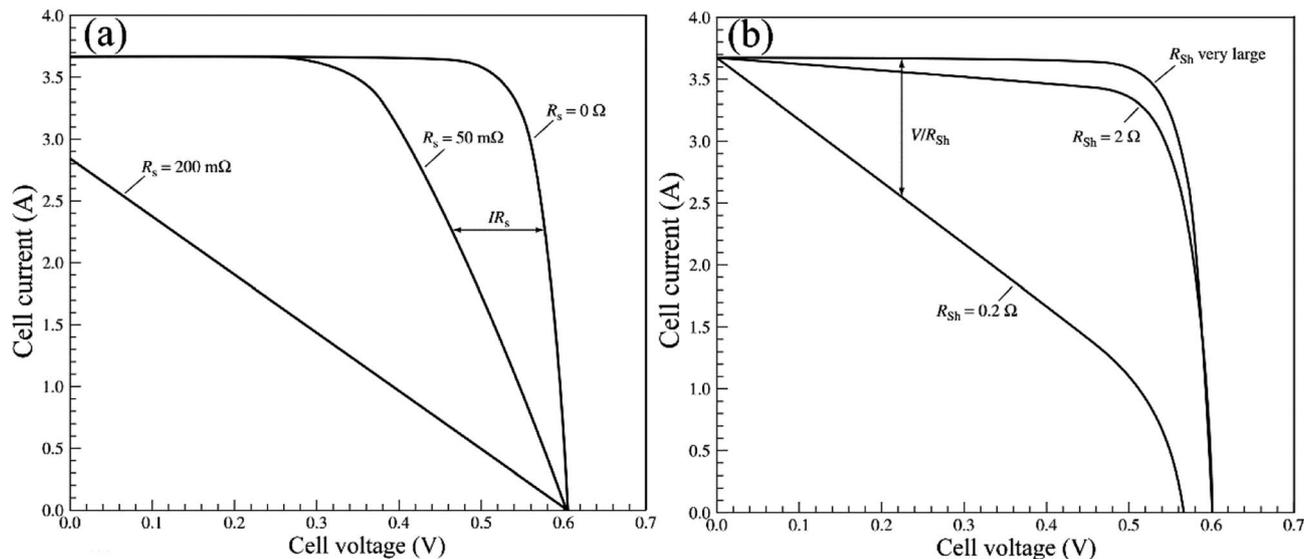
Fig. 18 (a)  $I$ - $V$  curve of  $R_s$ , (b)  $I$ - $V$  curve of  $R_{sh}$ .<sup>96</sup>
