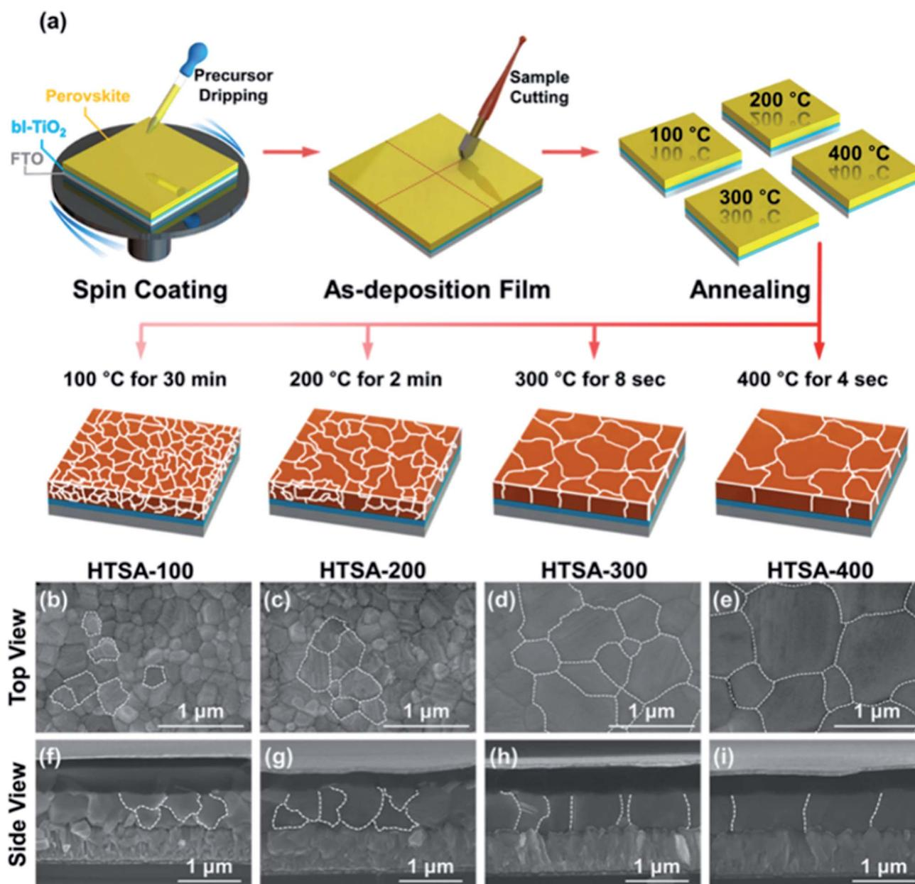
Fig. 7 (a) Schematic illustration of the annealing processes. (b–e) Surface SEM images (top view) of the perovskite films. (f–i) Their cross-sectional images (side view), respectively.<sup>35</sup>
