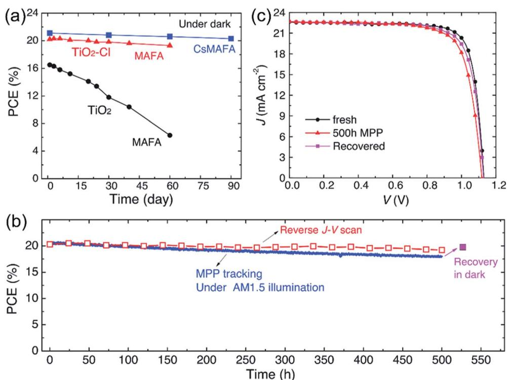
Fig. 25 Long-term device stability of PSCs with TiO<sub>2</sub>-Cl and TiO<sub>2</sub>. (a) Dark storage stability of non-encapsulated PSCs. (b) Continuous maximum power point tracking for 500 hours of a high performance unsealed CsMAFA cell with TiO<sub>2</sub>-Cl in nitrogen atmosphere under constant simulated solar illumination. (c) *J*-*V* curves of the PSCs (CsMAFA) from (b) at various stages.<sup>31</sup>
