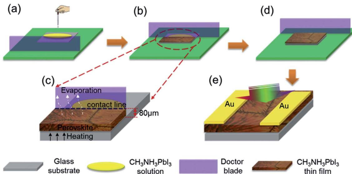
Fig. 15 Schematic representation of *in situ* doctor blading technology for fabricating CH<sub>3</sub>NH<sub>3</sub>PbI<sub>3</sub> films.<sup>22</sup>
