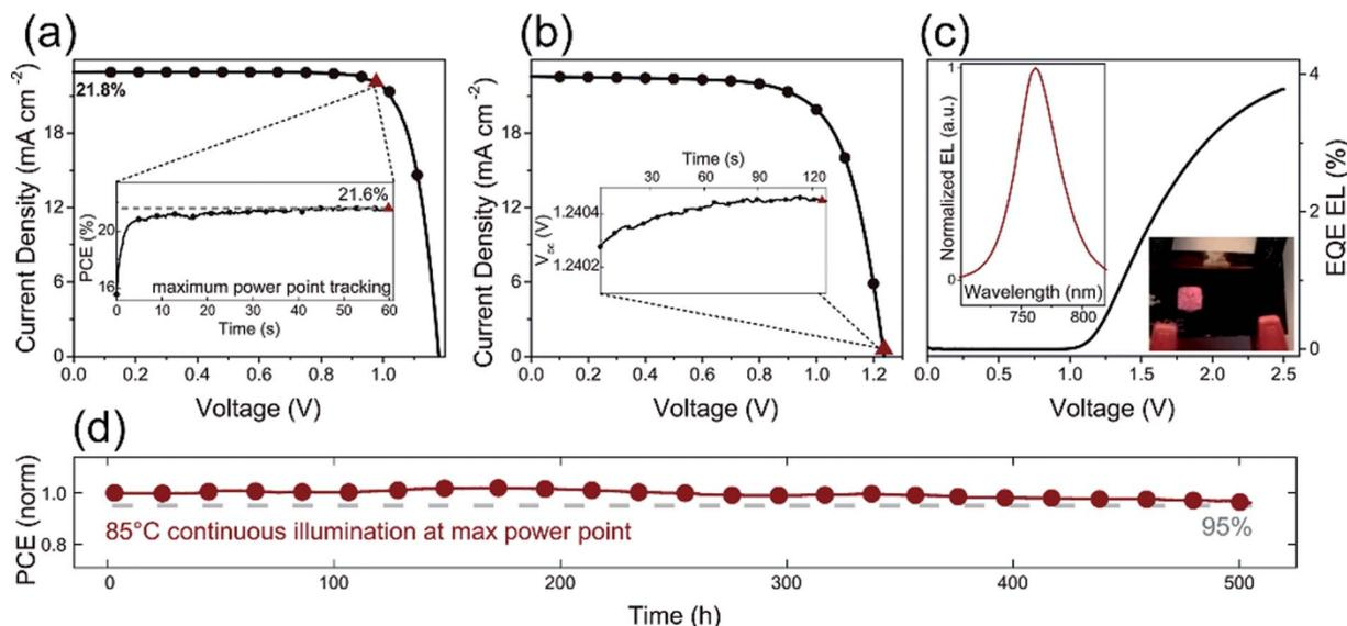
Fig. 26 (a)  $J$ - $V$  curve of RbCsMAFA solar cell. (b)  $J$ - $V$  curve of the highest- $V_{oc}$  device. (c) EQE electroluminescence (EL) as a function of voltage. (d) Thermal stability test of a perovskite solar cell.<sup>116</sup>
