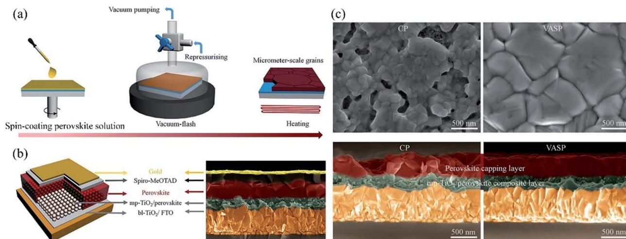
Fig. 8 (a) Schematic illustration of nucleation and crystallization procedures during the formation of perovskite film *via* VASP. (b) Schematic illustration of the PSCs configuration and SEM image. (c) Surface and cross-sectional SEM images of the perovskite films fabricated by the conventional process (CP) and VASP.<sup>37</sup>
