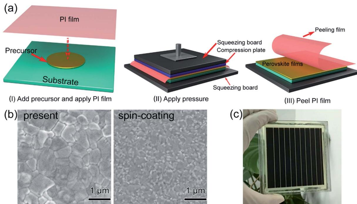
Fig. 14 Diagram of the pressure processing method for the deposition of perovskite films. (a) The steps of the pressure processing method. (b) SEM images. (c) Photograph of a perovskite module.<sup>36</sup>
