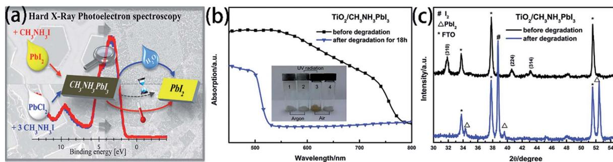
Fig. 22 (a) Degradation of MAPbI<sub>3</sub> in moisture and air atmosphere.<sup>109</sup> (b) UV-vis absorption spectra of TiO<sub>2</sub>/MAPbI<sub>3</sub> film before and after degradation.<sup>48</sup> (c) XRD patterns of TiO<sub>2</sub>/MAPbI<sub>3</sub> film before and after degradation.<sup>48</sup>
