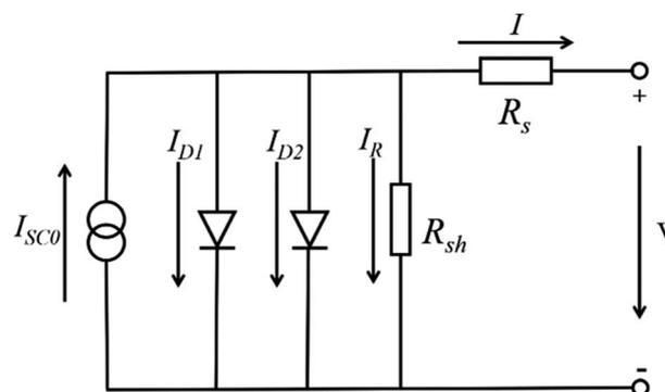
Fig. 17 Incorporating these resistances into the circuit model.<sup>96</sup>
