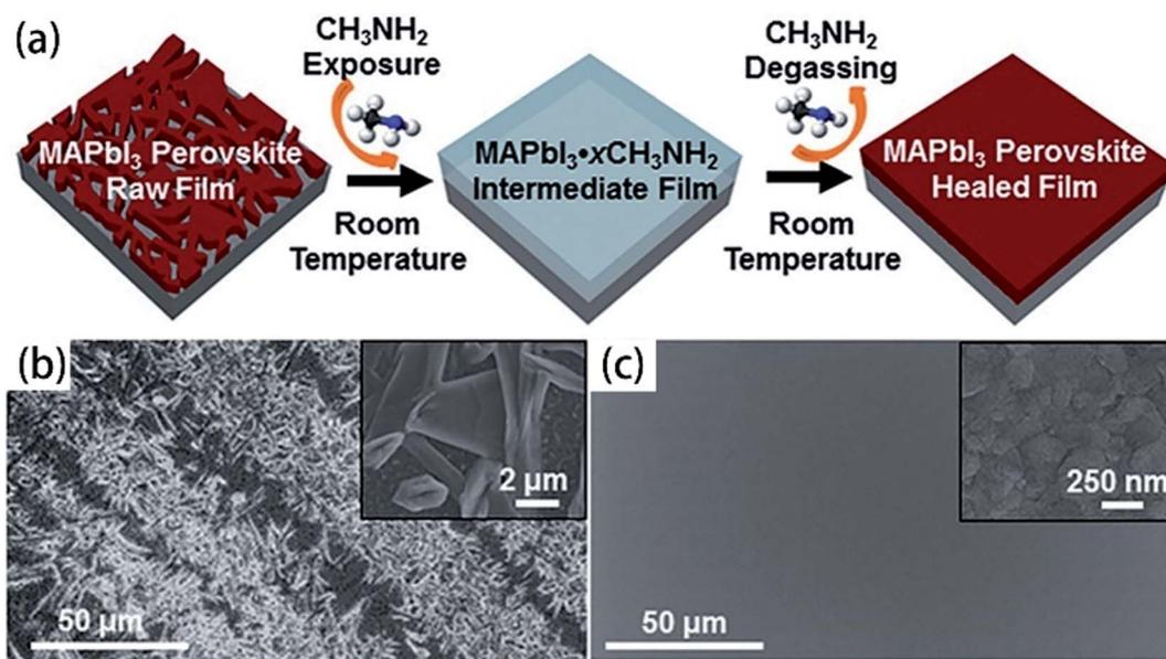
Fig. 12 (a) Schematic illustration of MA induced defect-healing of MAPbI<sub>3</sub> perovskite thin films. SEM images of MAPbI<sub>3</sub> thin films: (b) raw film and (c) healed film.<sup>93</sup>
