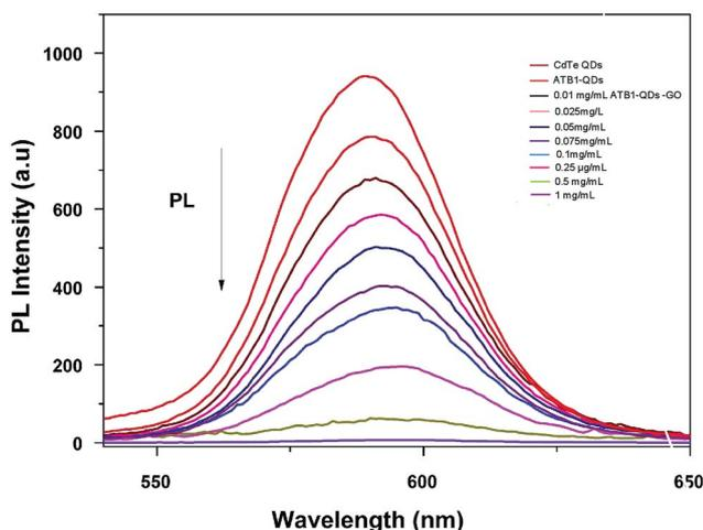
Fig. 5 Characterization of graphene oxide–quantum dots: monitoring the fluorescence quenching of quantum dots at various graphene oxide (0.01–1 mg ml<sup>-1</sup>) concentrations using PL spectroscopy.
