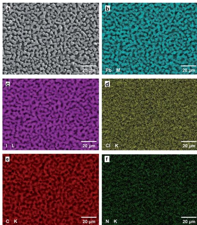
Fig. 6 (a) SEM image of the  $\text{CH}_3\text{NH}_3\text{PbI}_3(\text{Cl})$  cell containing 5 mg of  $\text{NH}_4\text{Cl}$ , and corresponding elemental mapping images of the (b) Pb M line, (c) I L line, (d) Cl K line, (e) C K line, and (f) N K line.
