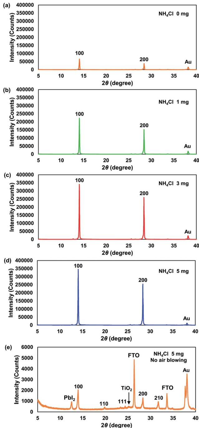
Fig. 7 XRD patterns of  $\text{CH}_3\text{NH}_3\text{PbI}_3(\text{Cl})$  cells containing (a) 0 mg, (b) 1 mg, (c) 3 mg, and (d) 5 mg of  $\text{NH}_4\text{Cl}$ , and (e) XRD pattern of the  $\text{CH}_3\text{NH}_3\text{PbI}_3(\text{Cl})$  cell containing 5 mg of  $\text{NH}_4\text{Cl}$  without air blowing.
