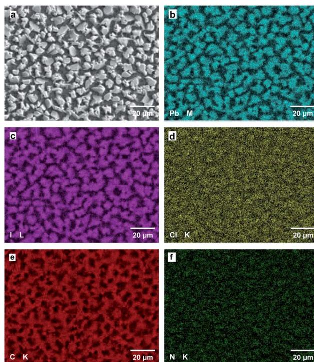
Fig. 5 (a) SEM image of the  $\text{CH}_3\text{NH}_3\text{PbI}_3(\text{Cl})$  cell without  $\text{NH}_4\text{Cl}$ , and corresponding elemental mapping images of the (b) Pb M line, (c) I L line, (d) Cl K line, (e) C K line, and (f) N K line.
