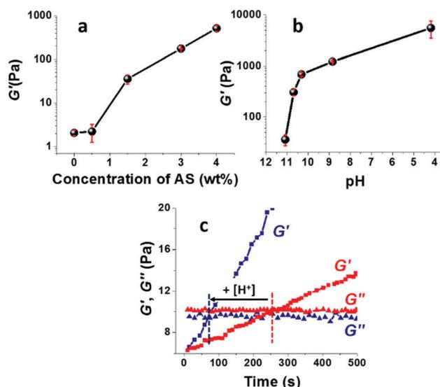
Fig. 3 Viscoelastic properties of the TCNF/AS dispersions and foams at room temperature. Storage modulus,  $G'$ , of TCNF/AS<sub>d</sub> as a function of (a) varying concentration of AS (pH 10.6–11.2) and (b) of TCNF/AS<sub>1.5\_d</sub> at different pH. (c) Evolution of the storage ( $G'$ ) and loss ( $G''$ ) moduli over time for TCNF/AS<sub>3\_wf</sub> at pH 11.1 (red) and pH 10.8 (blue) at room temperature, 1 min after foaming.
