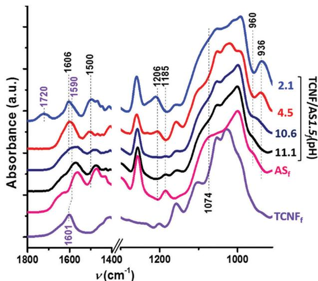
Fig. 4 ATR FTIR spectra of TCNF<sub>rd</sub>(pH 7), AS<sub>r</sub>(pH 10.5) and TCNF/AS<sub>1.5r</sub> at pH: 11.1, 10.6, 4.5 and 2.1 (labeled on the right of the graph).
