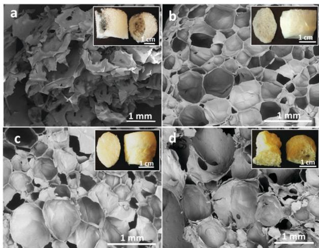
**Fig. 1** SEM images of the dry foam cross-sections: (a) TCNF/AS<sub>2f</sub>(11.1), (b) TCNF/AS<sub>4f</sub>(11.1), (c) TCNF/AS<sub>2f</sub>(10.8), (d) TCNF/AS<sub>2f</sub>(10.0). The insets represent the pictures of the corresponding dry foams.
