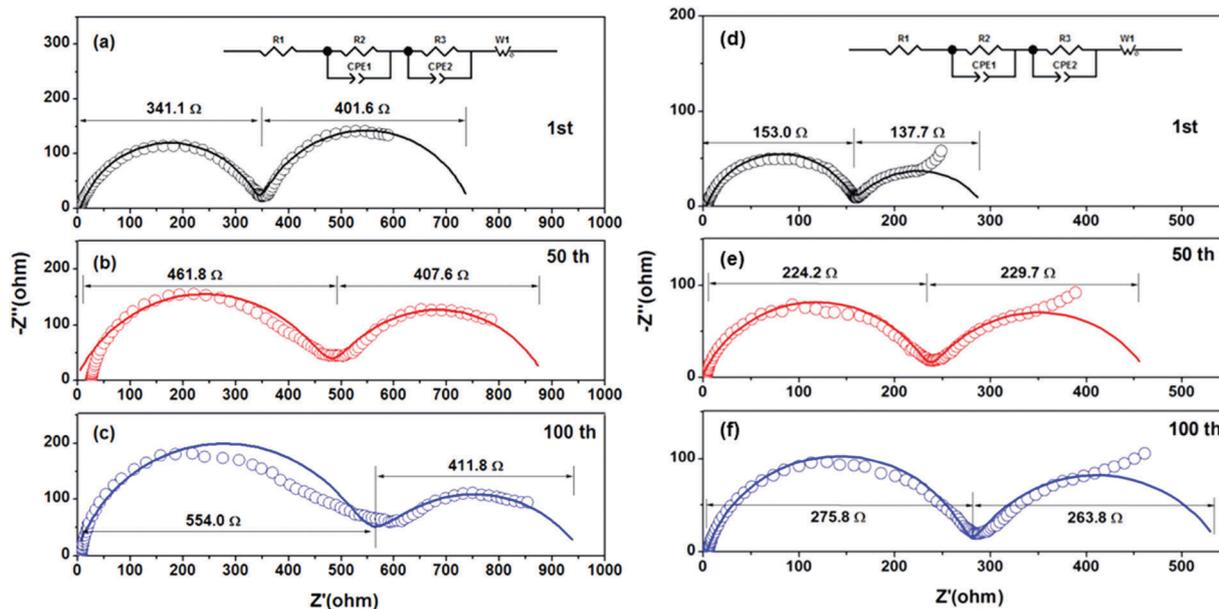
Fig. 6 EIS of  $\text{LiNi}_{0.8}\text{Co}_{0.1}\text{Mn}_{0.1}\text{O}_2$  prepared from (a–c)  $\text{Ni}_{0.8}\text{Co}_{0.1}\text{Mn}_{0.1}\text{O}_x$  and from (d–f)  $\text{Ni}_{0.8}\text{Co}_{0.1}\text{Mn}_{0.1}(\text{OH})_2@ \text{Ni}_{0.8}\text{Co}_{0.1}\text{Mn}_{0.1}\text{O}_x$  after different cycles: (a and d) 1st; (b and e) 50th; (c and f) 100th.
