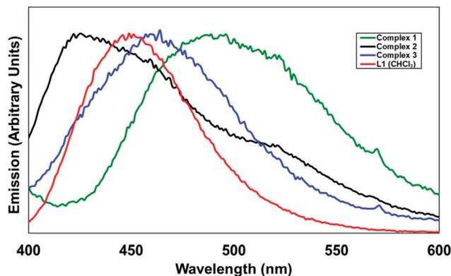
Fig. 10 Solid-state emission spectra for complexes **1–3**, compared with the emission of **L1** in  $\text{CHCl}_3$  solution (red).  $\lambda_{\text{ex}} = 366 \text{ nm}$  (**L1**) and  $380 \text{ nm}$  for the solids.
