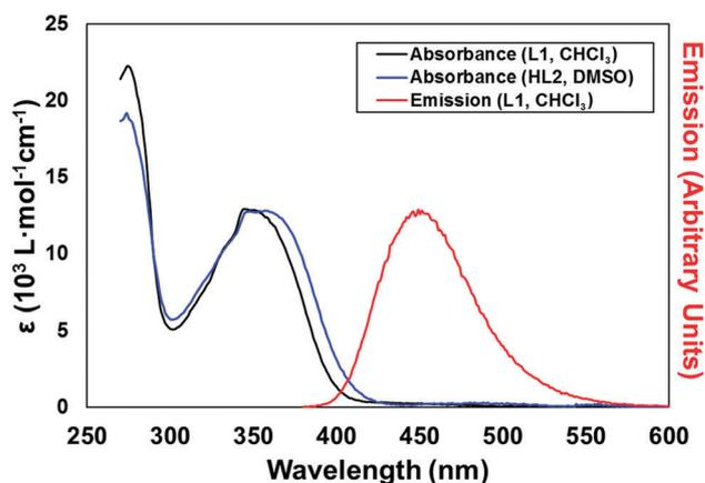
Fig. 2 Overlaid absorption spectra for **L1** and **HL2** (black and blue, respectively) and emission spectrum ( $\lambda_{\text{ex}} = 366 \text{ nm}$ ) for **L1**. All spectra were recorded at room temperature at 9  $\mu\text{M}$  concentration in  $\text{CHCl}_3$  (**L1**) or DMSO (**HL2**).
