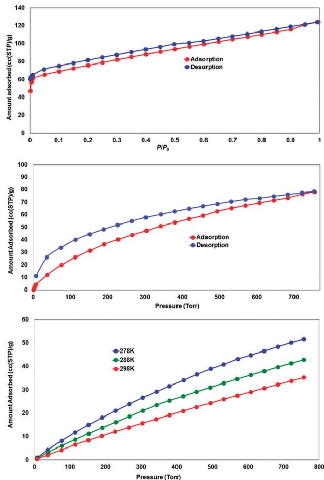
Fig. 9 Gas adsorption performance for the solvent-exchanged complex **4**, showing N<sub>2</sub> adsorption at 77 K (top), H<sub>2</sub> adsorption at 77 K (middle) and CO<sub>2</sub> adsorption at 278, 288 and 298 K (bottom).
