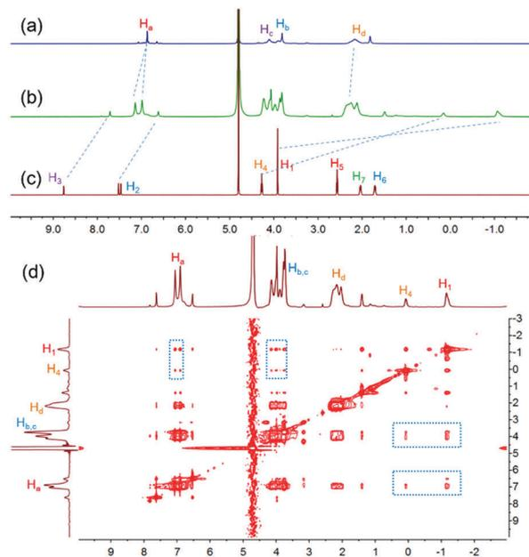
**Fig. 1** <sup>1</sup>H NMR spectra (400 MHz, D<sub>2</sub>O, 298 K): (a) **WP5-P** (10.0 mM); (b) **WP5-P** (10.0 mM) and **G1** (10.0 mM); (c) **G1** (10.0 mM). (d) 2D NOESY spectrum of a mixture of **WP5-P** (10.0 mM) and **G1** (10.0 mM). The NOE correlation signals that confirm the host-guest interactions are marked on the spectrum.
