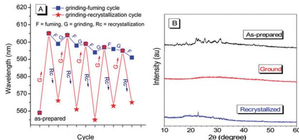
Fig. 29 (A) Variations of the emission wavelengths of **102** solids in grinding–fuming (blue trace) and grinding–recrystallization (red trace) cycles. (B) PXRD patterns for **102** of as-prepared microcrystal (upper), ground powder (middle) and re-crystallized samples (lower). Reproduced with permission from ref. 81. Copyright 2015 The Royal Society of Chemistry.
