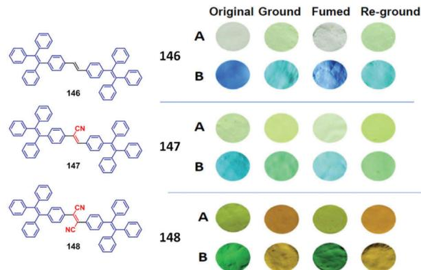
Fig. 40 (left) The molecular structures of compounds **146–148**. (right) Images of **146**, **147** and **148** samples (A) taken under natural light and (B) 365 nm UV-light with different processes: original sample, ground sample, fumed sample (obtained by fuming the ground sample in *n*-hexane vapor for 5 min), re-ground (ground sample of the above mentioned fumed sample). Reproduced with permission from ref. 105. Copyright 2015 The Royal Society of Chemistry.
