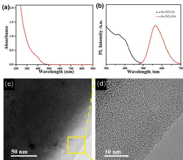
**Fig. 1** UV-vis absorption spectrum (a), photoexcitation ( $\lambda_{\text{em}} = 565$  nm, black line) and photoemission ( $\lambda_{\text{ex}} = 365$  nm, red line) spectra of the Au NCs (b). (c) TEM image of the Au NCs at pH 2.0. (d) HRTEM image of the zone marked by the yellow frame in (c).
