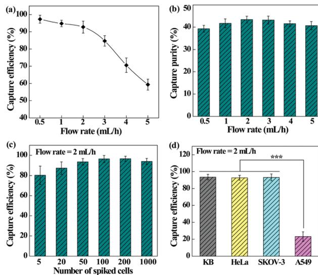
**Fig. 6** (a) Capture efficiency and (b) capture purity of HeLa cells at various flow rates. (c) Capture efficiency of HeLa cells after spiking of different numbers of HeLa cells with the WBCs. (d) Capture efficiency of different types of cancer cells under the same experimental conditions. In (a), (b), and (d), the cell densities of cancer cells and WBCs were 200  $mL^{-1}$  and 10<sup>6</sup>  $mL^{-1}$ , respectively.
