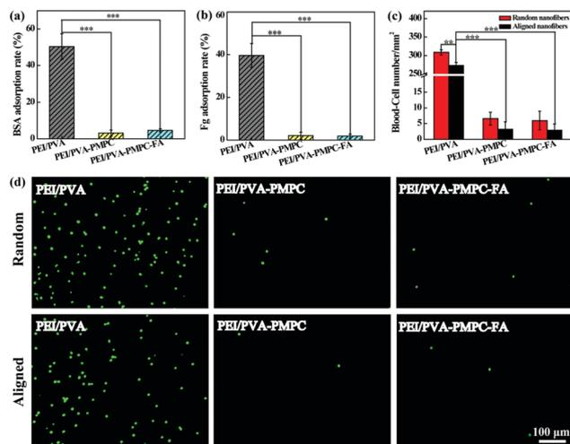
**Fig. 3** Adsorption rates of (a) BSA and (b) Fg on the aligned nanofibrous mats after incubation at 37 °C for 1 h. (c) The density of blood cells attached on the random and aligned nanofibrous mats. (d) Fluorescence microscopic images of WBCs attached onto different nanofibrous mats. A freshly isolated WBC suspension (1 mL,  $10^6 \text{ mL}^{-1}$ ) was added into each well and incubated at 37 °C for 1 h.
