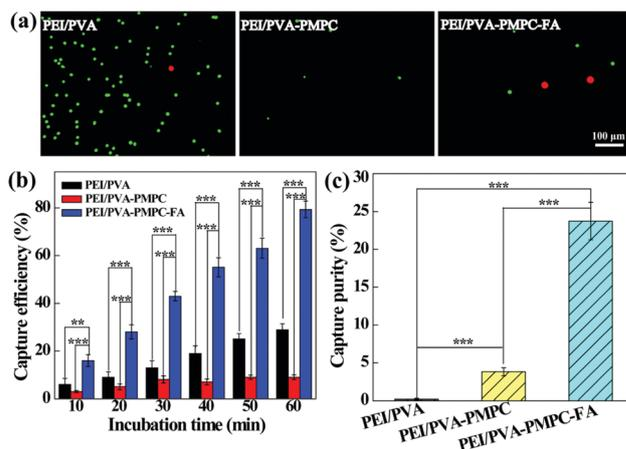
**Fig. 4** (a) Fluorescence microscopic images of HeLa cells (red) and WBCs (green) attached on different aligned nanofibrous mats after incubation for 1 h. (b) Capture efficiency of HeLa cells at various incubation time periods. (c) Capture purity of HeLa cells on different nanofibrous mats after incubation for 1 h. The HeLa cells were spiked into 1 mL of WBC suspension ( $10^6 \text{ mL}^{-1}$ ) with a HeLa cell density of  $200 \text{ mL}^{-1}$ .
