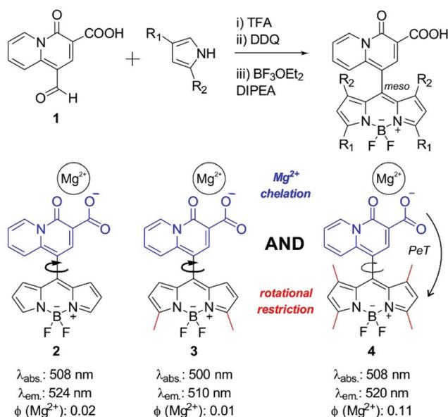
**Fig. 1** Simplified synthetic scheme for the preparation of Mg-sensitive BODIPY fluorophores based on the 4-oxo-4*H*-quinolizine-3-carboxylic acid chelating scaffold. Below are represented the chemical structures of BODIPY fluorophores **2**, **3** and **4** and their corresponding activation modes upon Mg<sup>2+</sup> recognition. Fluorescence quantum yields were determined relative to fluorescein in basic ethanol.
