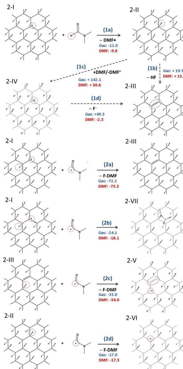
**Fig. 3** Radical mechanism of defluorination of FG in DMF. (1a–c) Initial phases of defluorination. (2a–d) Re-creation of FG radical center. The reaction energies are given in kcal mol<sup>-1</sup>.
