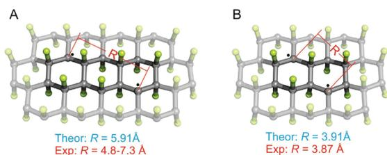
**Fig. 4** Structure of biradical sites on FG surface: typical biradical present on the FG surface (A); biradical 3-I observed in the later phases of the defluorination process (B). The experimental distances were estimated from the analysis of EPR spectra (see section 3.1).
