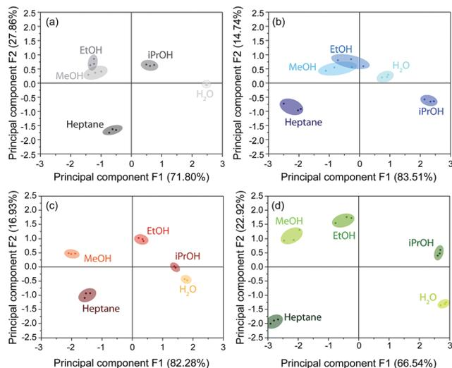
**Fig. 6** PCA score plots for (a) CAU-1, (b) CAU-1-SBU and (c) CAU-1-Hex visualizing the discrimination capability of the BSs towards the solvent vapors of water, methanol, ethanol, iso-propanol and heptane; (d) PCA plot for a combined array of the pristine and modified BSs. Different color scales are used for clarity. The percentages of variance of the principal components F1 and F2 are given in brackets.
