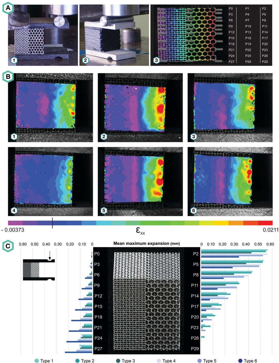
**Fig. 3** Hybrid meta-biomaterials. (A) Test set-ups and image processing: (1) off-axis compression, (2) off-axis compression with an adherent layer used to improve visualization of strain distribution, (3) points plotted along the borders of a hybrid meta-biomaterial and the order in which they were numbered according to their position. (B) Horizontal strains in the tape surrounding hybrid meta-biomaterials types 1–6 at 2 mm displacement. (C) Mean maximum expansion during off-axis compression.
