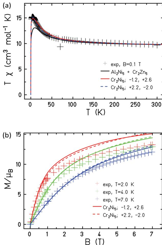
Fig. 12 Experimental and simulated magnetic susceptibility (a) and magnetisation (b) of **1**. The solid coloured curves belong to the parameterization  $J_{\text{Cr-Ni,r}} = -1.2 \text{ cm}^{-1}$ ,  $J_{\text{Cr-Ni,c}} = 2.6 \text{ cm}^{-1}$ , whereas the dashed ones belong to  $J_{\text{Cr-Ni,r}} = 2.2 \text{ cm}^{-1}$ ,  $J_{\text{Cr-Ni,c}} = -2.0 \text{ cm}^{-1}$ .
