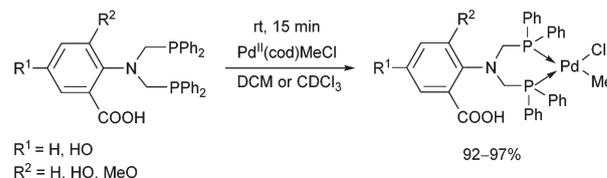
**Scheme 24** Preparation of mononuclear Pd<sup>II</sup> complexes from  $\alpha$ -aminophosphines bearing a benzoic acid moiety.
