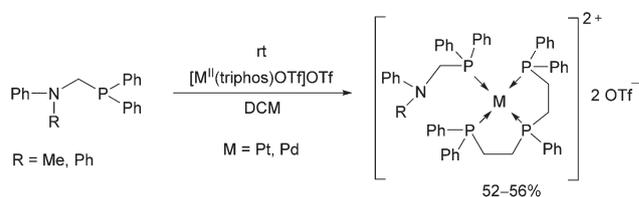
**Scheme 10** Synthesis of [Pt(triphos)P(Ph)<sub>2</sub>CN(Ph)(R)](OTf)<sub>2</sub> complexes.
