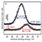
Fig. 19 Experimental Mg 2p XPS spectra of 14 ML and 1 ML MgO/Ag(100). Adapted from ref. 229. Copyright 2011 Wiley-VCH.
