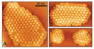
Fig. 26 STM images of the  $FeO_{2-x}$  islands after exposure to  $10^{-6}$  mbar CO at 400 K for 4 min. Tunneling conditions: bias -3 V, current 0.05 nA. The arrows highlight non-uniform disappearance of the Moiré spots close to the island edge.<sup>272</sup> Reproduced with permission from ref. 272. Copyright 2015 Wiley-VCH.
