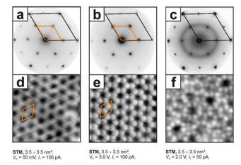
**Fig. 10** Low energy electron diffraction diagrams and STM topographic images of the respective systems, *i.e.* (a) and (d) a silica monolayer on Ru(0001), SiO $_{2.5}$ /Ru(0001), (b) and (e) a crystalline bilayer and (c) and (f) a vitreous (amorphous) bilayer, SiO $_2$ /Ru(0001). <sup>163,166</sup> Adapted with permission from ref. 166. Copyright American Chemical Society, 2012.
