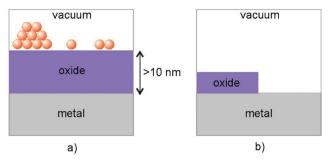
Fig. 17 Schematic illustration of (a) a "regular" model system and (b) one representing an "inverse" catalyst. Adapted with permission from ref. 208. Copyright 2016 American Chemical Society.
