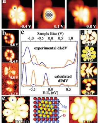
Fig. 13 (a) STM topographic and (b) conductance images of a Au<sub>18</sub> cluster on 2 ML MgO/Ag(001) ( $I_t = 5$  pA,  $3.9 \times 3.9$  nm<sup>2</sup>) in comparison with simulated (d) conductance and (e) topographic images (2.0  $\times$  2.0 nm²) and a structure model. (c) Experimental and simulated dI/dV spectra recorded at the blue and orange dots marked on the cluster in (a) and (e). Reprinted with permission from ref. 38. Copyright 2009 by the American Physical Society.
