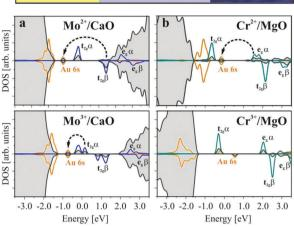
Fig. 8 Top: STM topographic images of Mo-doped and Cr-doped MgO(001) films. Bottom: Projected densities of states (DOS) for (a)  $CaO_{Mo}$ and (b) MgO<sub>Cr</sub> in the presence of a Au atom calculated for two different charge states of the transition metal ion. Charge-transfer processes from the HOMO of the dopant to the Au 6s affinity levels are indicated by arrows.  $^{\rm 120}$  Reproduced with permission from ref. 120. Copyright American Chemical Society, 2012.
