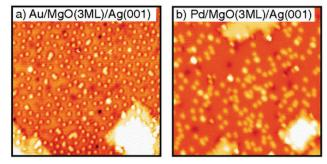
Fig. 11 STM images (30  $\times$  30 nm<sup>2</sup>) of (a) Au atoms ( $\theta$  = 2.9% ML Au) adsorbed on 3 ML thin MgO films ( $V_s = 0.5 \text{ V}$ ,  $I_t = 11 \text{ pA}$ ); and (b) Pd atoms ( $\theta = 2.3\% \text{ ML}$ Pd) adsorbed on 3 ML thin MgO films ( $V_s = 0.2 \text{ V}$ ,  $I_t = 13 \text{ pA}$ ). Reprinted with permission from ref. 195. Copyright 2007 by the American Physical Society.
