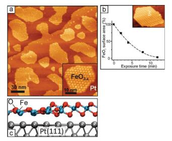
Fig. 25 (a) Typical morphology of oxidized  $FeO_{2-x}$  films on Pt(111) at submonolayer coverages. The cross-view of a FeO<sub>2-x</sub>/Pt(111) film is shown in the inset. (b) The  $FeO_{2-x}$  surface area normalized to the area in the "as prepared" sample as a function of the accumulative exposure time.  $^{272}$  (c) Schematic based on calculations of the FeO/FeO<sub>2-x</sub> interface after ref. 265. Copyright 2015 Wiley-VCH.
