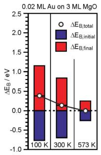
Fig. 15 Graphical representation of the EB-shifts derived from XPS and Auger measurements for 0.2 ML Au on 30 ML MgO(001)/Ag(001) with reference to Au(111).181
