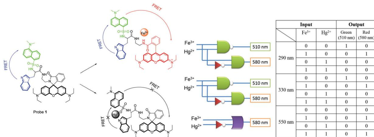
Fig. 9 Proposed binding mechanisms of the probe with Fe<sup>3+</sup> and Hg<sup>2+</sup> and the truth table.
