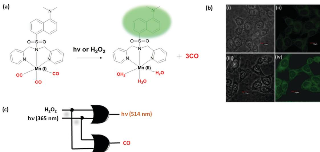
**Fig. 16** Two OR logic gates generated through light and hydrogen peroxide mediated CO release. (a) Chemical structure of a CO-releasing Mn complex. (b) Confocal microscopy images of HCT116 colon cancer cells: (i and iii) bright-field images, (ii) image without illumination, and (iv) image illuminated with 405 nm LED light. (c) Logic gate diagram. Reproduced with small alterations from ref. 31 with permission from Royal Society of Chemistry, copyright 2017.
