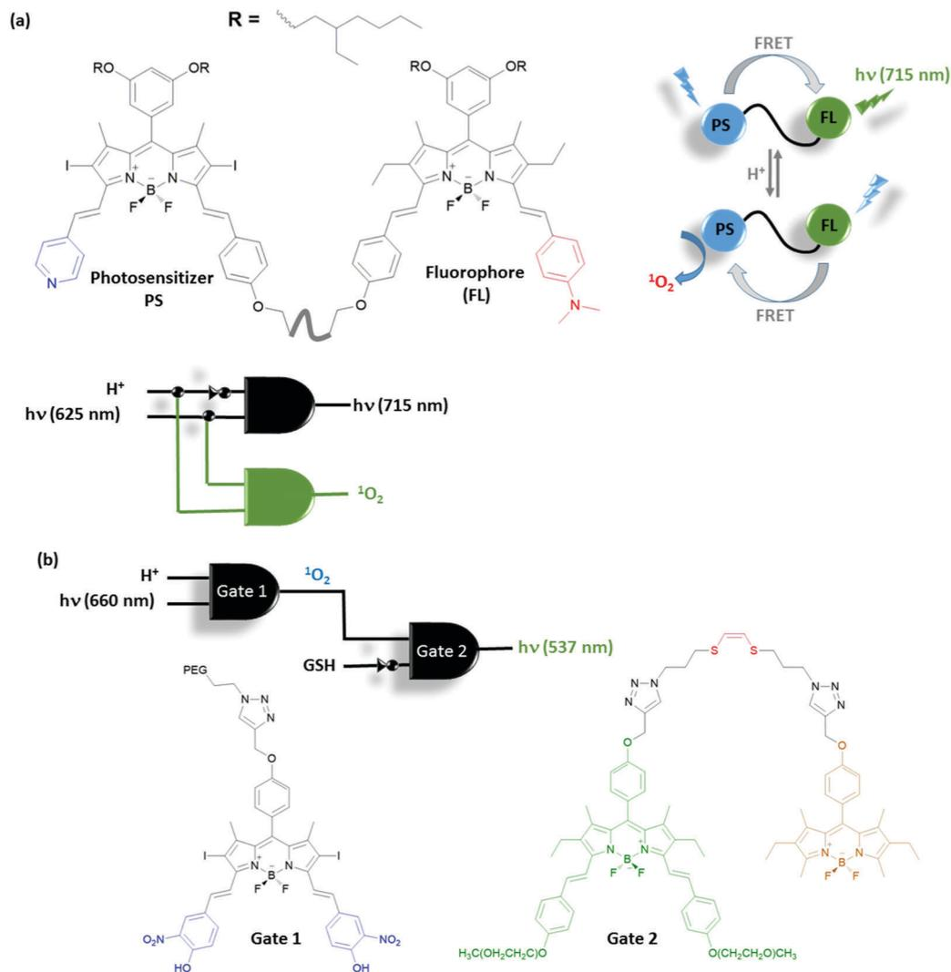
Fig. 19 Smart photosensitizers with higher order logic operations or a concatenated gate having potential biological function. (a) A molecular demultiplexer switching between therapy and diagnosis as it changes the direction of energy transfer taking place between modules, and (b) concatenated logic gates assembled within a micelle that enables fluorescence activity reporting of an acid activatable photosensitizer. PEG: polyethylene glycol.
