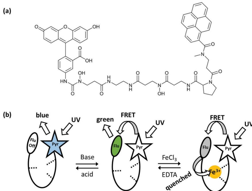
Fig. 5 (a) Molecular structure that can operate as a half-adder and half-subtractor depending on the choice of inputs and outputs. (b) Three different fluorescence states of the molecular logic gate. Reproduced from ref. 7 with permission from American Chemical Society, copyright 2004.
