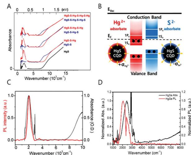
Fig. 4 (A) Absorption spectra of HgS CQD with S<sup>2-</sup> and Hg<sup>2+</sup> layer by layer growth. Reprinted with permission from ref. 36 copyright 2014 American Chemical Society. (B) Surface treatment schematics of HgS CQD (C) HgS absorption and photoluminescence spectra reprinted with permission from ref. 39. Copyright 2014 American Chemical Society. (D) HgSe absorption and photoluminescence.
