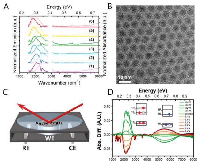
**Fig. 11** Ag<sub>2</sub>Se CQD absorption and photoluminescence (A) and TEM image (B). The schematics of spectro-electro chemical cell (C) and reduction (green) and oxidation (red) spectra of Ag<sub>2</sub>Se sample (D). Adapted with permission from ref. 69. Copyright 2018 American Chemical Society.
