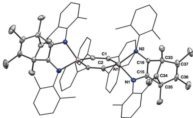
Fig. 3 Solid state structure of **2** determined by single crystal X-ray diffraction. Ellipsoids are at 50% probability. Phenyl and 2,6-dimethylphenyl groups are drawn in wireframe and hydrogen atoms are omitted for clarity. Selected bond lengths (Å) and angles (°) = Al1–C2 1.977(7), Al1–C1 1.981(7), Al1–N1 1.946(6), Al1–N2 1.949(6), C15–C16 1.401(10), C36–C37(11), C15–C34 1.988(11), C16–C34 1.962(11), C34–C33–C16 79.8(5), C34–C33–C15 81.6(5).
