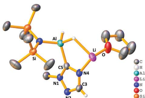
**Fig. 5** Asymmetric unit of polymeric structure of **9** with triazole ring atoms labelled. Hydrogen atoms (except hydride and C3–H) and disordered THF molecules have been omitted for clarity. Thermal ellipsoids are drawn at 40% probability.
