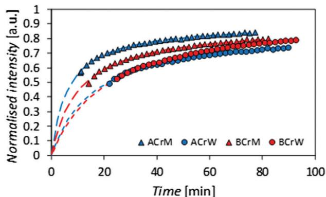
Fig. 4 Recovery of fluorescence intensity for regenerated cellulose hydrogels after bleaching. A more rapid recovery is observed in the methanol regenerated samples and those generated from  $\alpha$ -cellulose.
