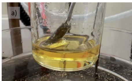
Fig. 1 (a) Liquid monosaccharide-urea melt obtained from glucose.
