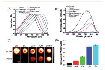
Fig. 1 The spectroscopic and PA responses of ER-P in various solvents with different polarity indices. (A and B) The absorption and fluorescence spectra of ER-P (10 µM, 1% DMSO as a cosolvent) in seven solvents with different polarities. (C and D) Representative PA images and PA intensity ratios of ER-P (50  $\mu$ M, 1% DMSO as a cosolvent) in five solvents with different polarities. Dio, dioxane; EA, ethyl acetate; DCM, dichloromethane; ACN, acetonitrile; DMSO, dimethyl sulfoxide.
