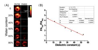
Fig. 2 (A) Representative PA images of ER-P (10 μM, 1% DMSO as a cosolvent) with excitation at 700 and 800 nm in dioxane-water mixtures (water from 0 to 80%). (B) The linear relationship between the PA intensity ratios of ER-P (10 μM) and dielectric constant.
