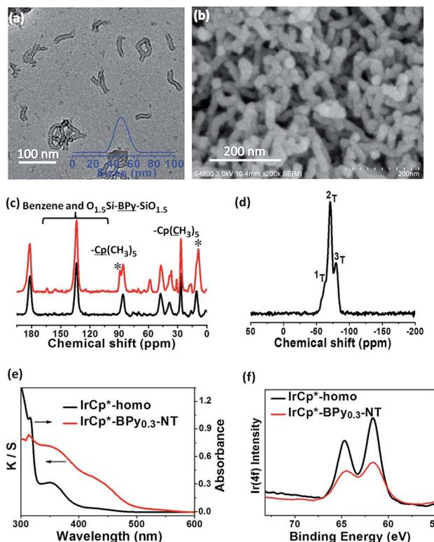
Fig. 2 (a) TEM and (b) SEM images of  $\text{IrCp}^*\text{-BPY}_{0.3}\text{-NT}$ . (c)  $^{13}\text{C}$  CP MAS NMR spectra of  $\text{BPY}_{0.3}\text{-NT}$  (black line) and  $\text{IrCp}^*\text{-BPY}_{0.3}\text{-NT}$  (red line). (d)  $^{29}\text{Si}$  MAS NMR spectrum of  $\text{IrCp}^*\text{-BPY}_{0.3}\text{-NT}$ . (e) UV/vis diffuse reflectance spectra and (f) XPS spectra of  $\text{IrCp}^*\text{-homo}$  (black line) and  $\text{IrCp}^*\text{-BPY}_{0.3}\text{-NT}$  (red line).
