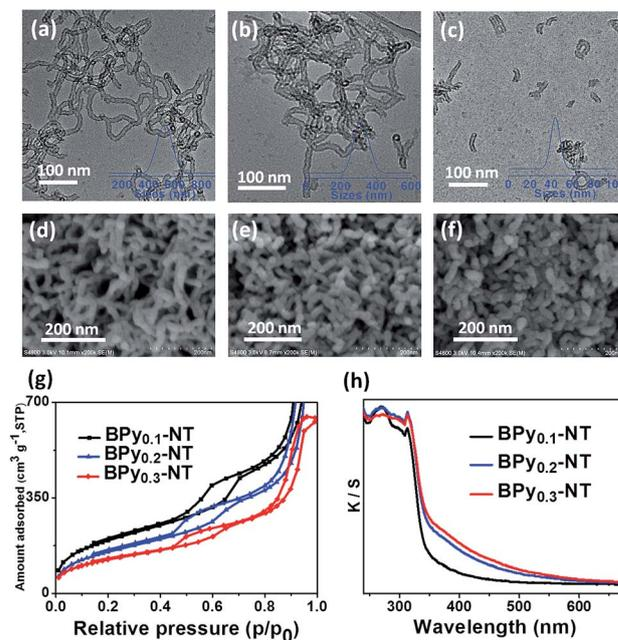
Fig. 1 (a–f) TEM and SEM images of (a and d) BPy<sub>0.1</sub>-NT, (b and e) BPy<sub>0.2</sub>-NT, and (c and f) BPy<sub>0.3</sub>-NT, respectively. Insets in (a–c) are the nanotube length distribution in ethanol obtained *via* dynamics light scattering. (g) Nitrogen adsorption–desorption isotherms and (h) UV/vis diffuse reflectance spectra of BPy<sub>0.1</sub>-NT (black line), BPy<sub>0.2</sub>-NT (blue line), and BPy<sub>0.3</sub>-NT (red line).
