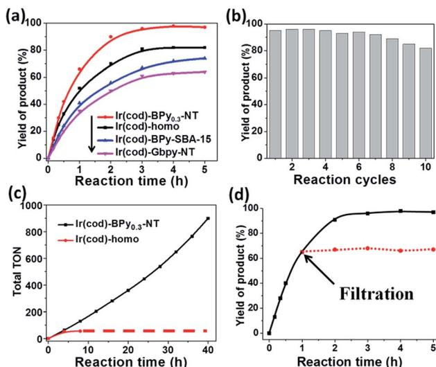
Fig. 6 (a) Reaction kinetic curves of benzene borylation catalyzed by Ir(cod)-homo (black line), Ir(cod)-BPy<sub>0.3</sub>-NT (red line), Ir(cod)-BPy-SBA-15 (blue line), and Ir(cod)-Gbpsy-NT (pink line). (b) Reusability of Ir(cod)-BPy<sub>0.3</sub>-NT for benzene borylation. (c) Total TONs of Ir(cod)-BPy<sub>0.3</sub>-NT (black line) and Ir(cod)-homo (red line) for the recycling. (d) Filtration experiment of Ir(cod)-BPy<sub>0.3</sub>-NT catalyst (red-dotted line).
