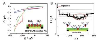
Fig. 5 Studying the single HRP with a BLM-Au nanoelectrode.<sup>6</sup> (A) Cyclic voltammograms of the BLM-Au nanoelectrode (1) and HRPembedded BLM-Au nanoelectrode (2) in a solution of 20 mM H<sub>2</sub>O<sub>2</sub> and PBS buffer (pH: 7.4). (B) Chronoamperometric response of HRP collision into the BLM-Au electrode.6 Reproduced by permission of ref. 6 from The Royal Society of Chemistry.
