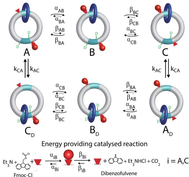
Fig. 2 Kinetic cycle for the molecular motor described by Wilson *et al.*<sup>8</sup> The deuterated recognition site serves as a fiduciary marker for determining directionality but does not otherwise influence the kinetics or thermodynamics of the motor.
