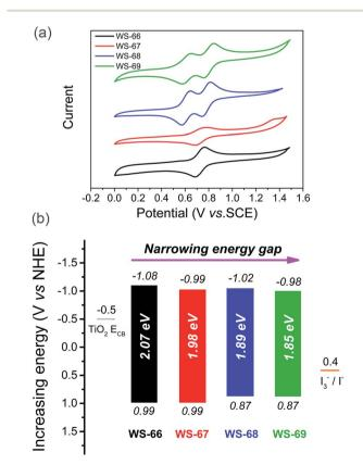
Fig. 3 Cyclic voltammograms of dyes WS-66, WS-67, WS-68 and WS-69 measured in  $CH_2Cl_2$  (a), LUMO (above the coloured bar) and HOMO (under the coloured bar) values, and energy band gaps of dyes WS-66, WS-67, WS-68 and WS-69 (b).
