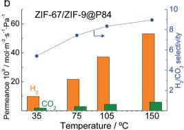
Fig. 6 Double-layered ZIF-8/ZIF-9 (a) and ZIF-67/ZIF-9 (b) membrane permeation properties in the  $\rm H_2/CO_2$  mixture separation as a function of temperature.
