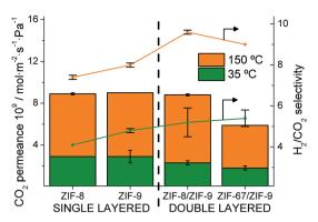
Fig. 5  $CO_2$  permeance and  $H_2/CO_2$  separation selectivity for single and double-layered ZIF@P84 membranes at 35 °C (green) and 150 °C (orange).
