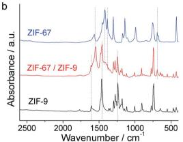
Fig. 4 XRD (a) and FTIR (b) spectra of the ZIF powders collected during the microfluidic syntheses. ZIF-8 with Zn and the Co-based ZIF-67 and ZIF-9 crystallize with the sod-structure. XRD spectrum of the double-layered ZIF@P84 HF membranes is also shown.
