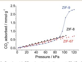
Fig. 2 Experimental  $CO_2$  adsorption isotherms at 25 °C of the powdered cobalt-based materials ZIF-9 (blue triangles) and ZIF-67 (red circles), compared with the ZIF-8  $CO_2$  isotherm (black squares) reported by Zornoza *et al.*<sup>56</sup> Solid lines show simulated ZIF-8 (black) and ZIF-67 (red) isotherms with a good fit to the experimental data (filled symbols). The solid line in the ZIF-9 isotherm is a guide to the eye.
