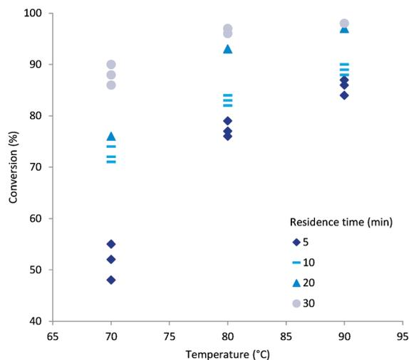
Fig. 3 Conversion (%) versus temperature (C) using high acrylic acid (1) concentration (1 mM) and low initiator (2) (1.25 mol%) input.
